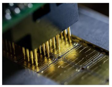
Fig. 7: Production of a security smartcard chip module with T-Systems' TCOS operating system
